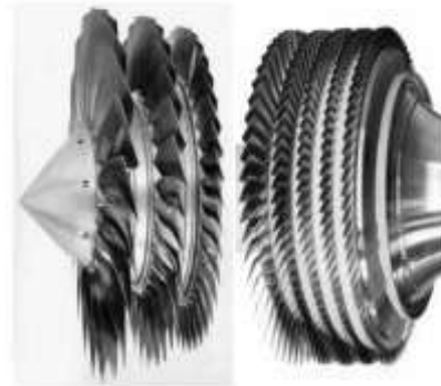
Fig 1 Transonic lpc (left) and hpc (right) eurofighter typhoon engine EJ200
