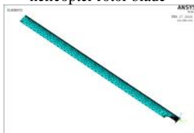
Fig shows the finite element model of helicopter rotor blade
