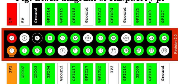
Fig: Pin description of Raspberry pi
