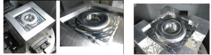
(a) Cavity contour milling (b) variable contour milling (c) Five-axis positioning milling result
