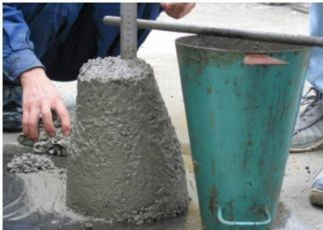
Figure 3: Highly workable fresh concrete
