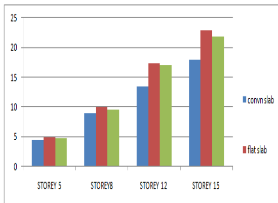
Fig:39: Story displacement Graph Between Flat Slab, Flat Slab With Perimeter Beams And Conventional Slab In Zone II in soil-I
