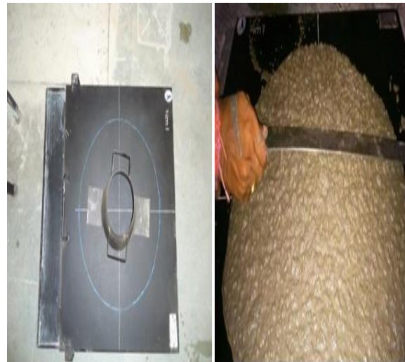
Fig. Slump Flow Apparatus & Testing
