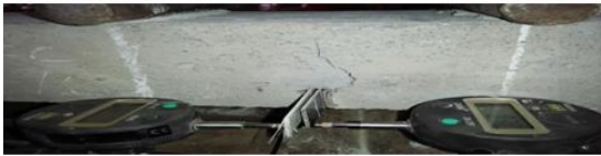
Fig. 4.6.2 Crack Pattern of GFC-1
