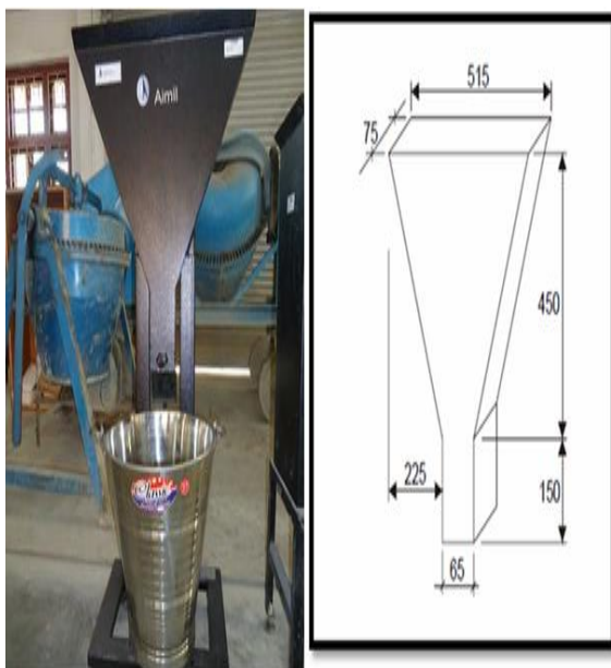
Fig. V-Funnel Apparatus and Schematic Diagram
