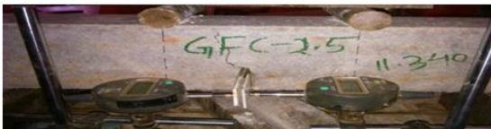
Fig.4.6.4 Crack Pattern of GFC-2.5
