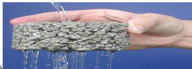
Figure 1.2 Pervious Concrete block
