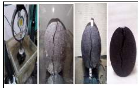
Figure 10. Loading and failure pattern of indirect tensile strength test
