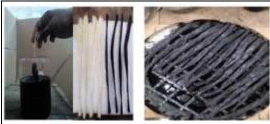
Figure.7.Coating of emulsion on Fibre and Oven dry Fibre
