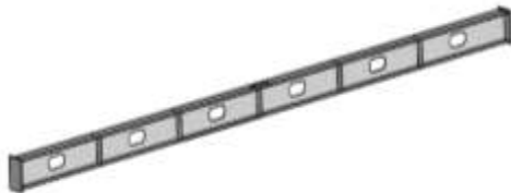
Slot Shape Web opening Beam (Slot size – 100 x 200)
