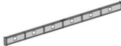
Rectangular Shape Web Opening Beam (Rectangle Size – 100 x 150)
