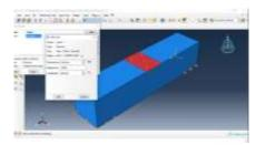
2. Plain cement concrete beam with Glass fiber plates.
