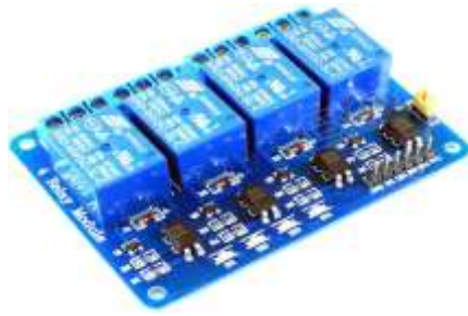
Figure.3: Relay Driver Module
