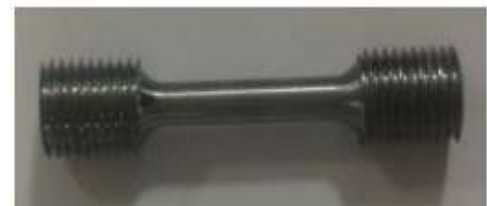
Figure 2 specimen of P265GH steel material according to ISO 6892 [3].
