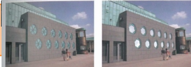
Fig 11: Potential transformable facade utilizing a simpler swivel diaphragm CONCEPTUAL DESIGN (5)
