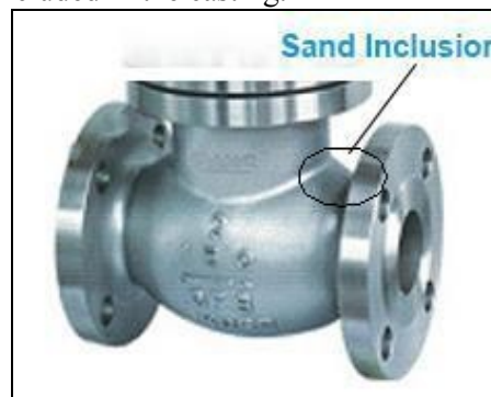
Figure 1 Sand inclusion in valve casting
