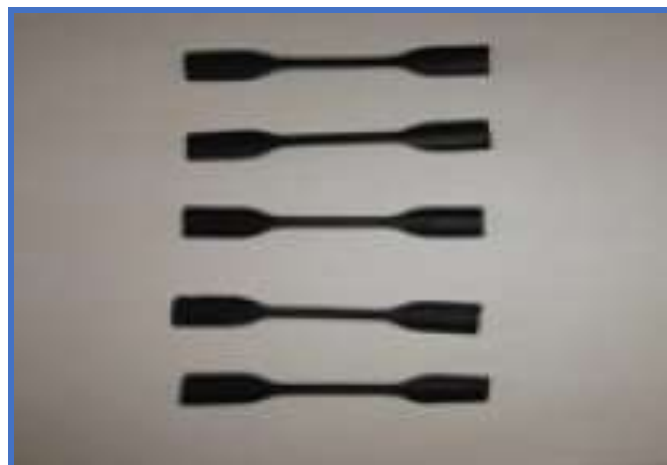
Figure 2 specimen of PR and PVC material according to ISO 6892 [3].
