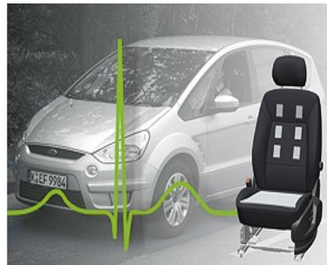
Fig .6. Electrodes attached to the seat of the drivers
