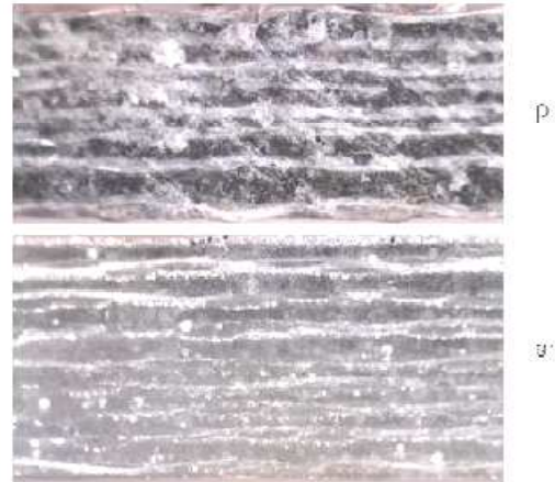
Figure 11. The microscopic views of the composite material without recycled rubber and with recycled rubber are as shown in the figure.
