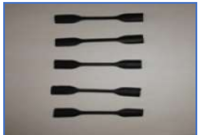
Figure 2 specimen of PR and PVC material according to ISO 6892 [3].
