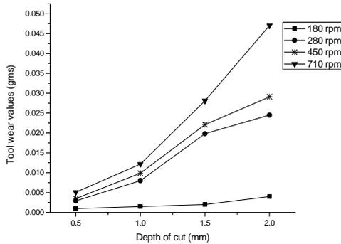
Figure 11. Tool wear values for turning
