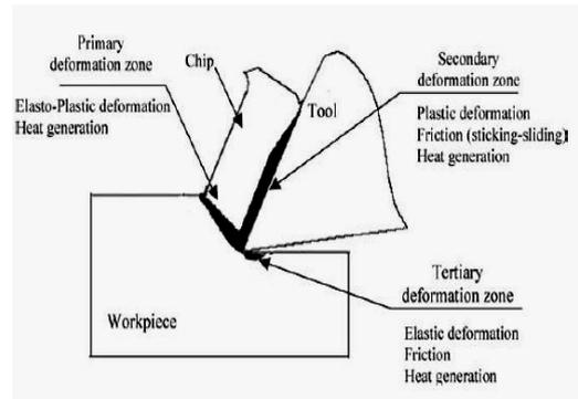
**Figure 1.** Sources of heat generation in the orthogonal cutting process [5].
