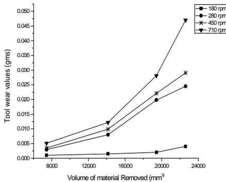
Figure 12. Tool wear Vs Volume of material removed
