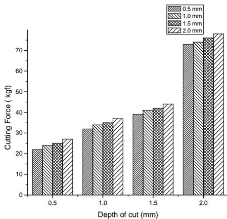
Figure 8. Tangential force (F<sub>y</sub>) Values
