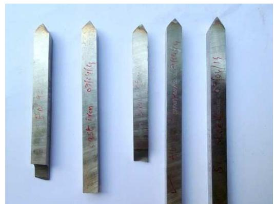
Figure 3. HSS Tool Used for Tests
