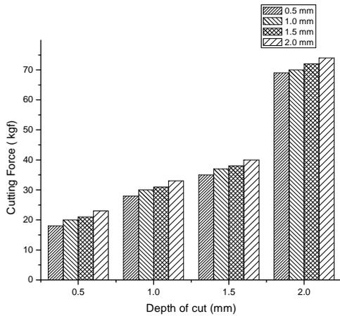
Figure 7. Cutting force (F<sub>x</sub>) Values
