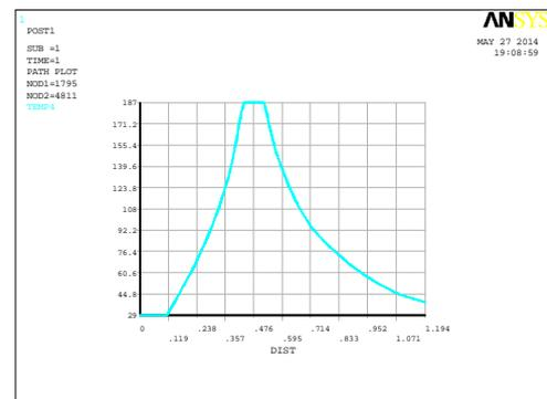
Figure 17. Temperature Distribution at Machining interface
