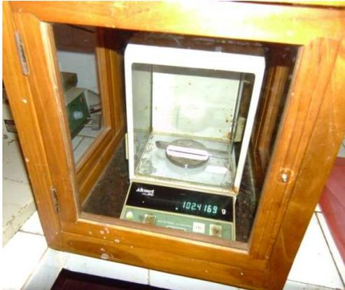
**Figure 4.** Electronic Balance (Lc= 0.0001gm)
