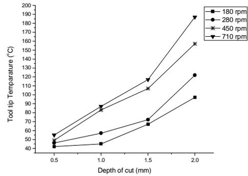
Figure 10. Temperature developed in Turning
