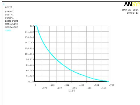
**Figure 18.** Temperature Distribution over tool tip surface
