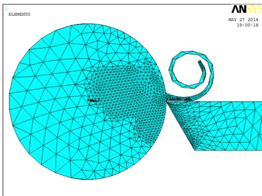
Figure 15. Tool work Model meshed Elements
