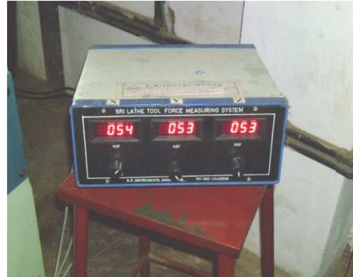
**Figure 6.** Tool dynamometer Output
