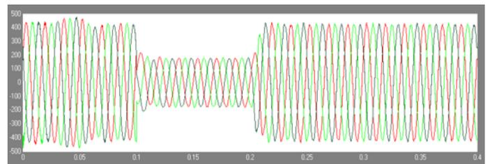
Fig. 17 System during 3-phase fault
