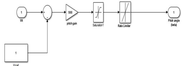
Fig. 6 Pitch Angle Controller Model
