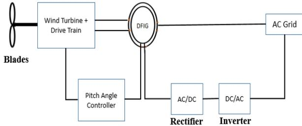
Fig. 1 DFIG based on wind energy conversion system
