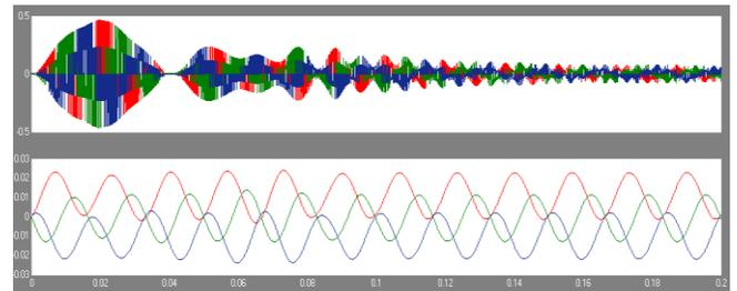
Fig. 16 Rotor voltage and current waveform
