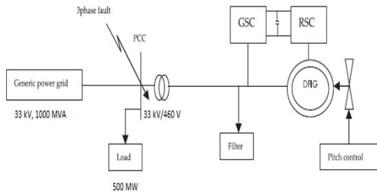
Fig. 8 Single line diagram for the system
