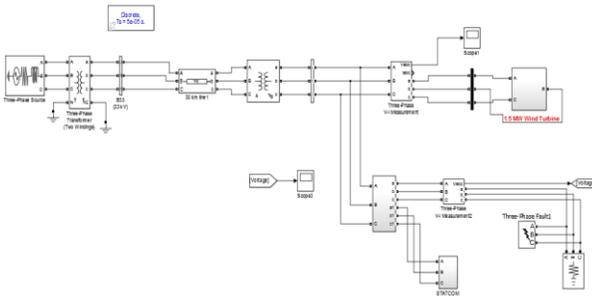
Fig. 12 Grid connected DFIG with STATCOM
