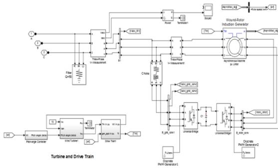
Fig. 7 DFIG with its converters
