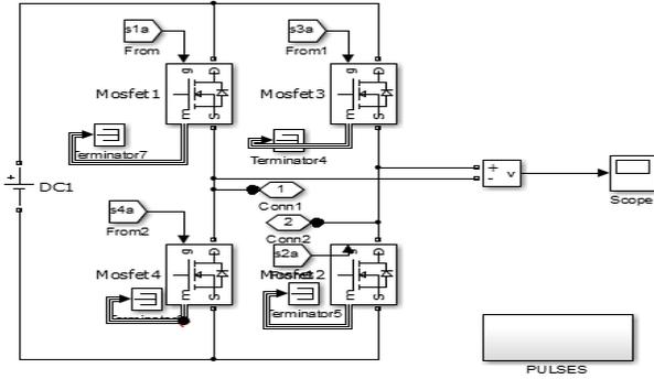
Fig. 11 Multilevel Inverter
