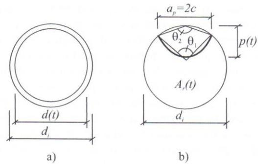
**Figure 2: a) uniform corrosion b) pitting corrosion**
