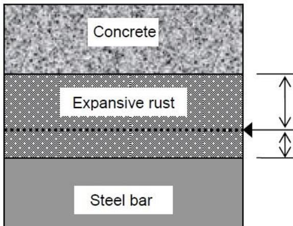
**Figure 1** Schematic illustration of corroding rebar and expansive rust: 50 μm section loss of steel. Rust volume is three times that of the corroded steel (150 μm)
