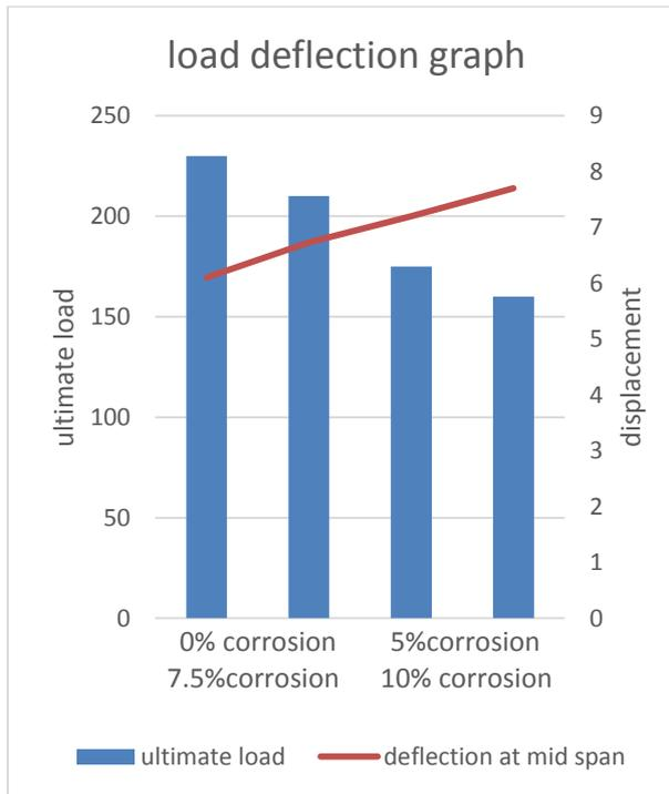
**Figure 4.1: load vs deflection value of all models**
