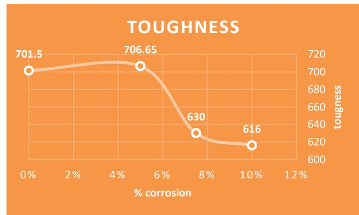
**Figure 4.3: Toughness Vs corrosion**
