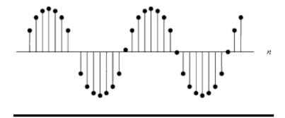
A signal x(t) is discrete time signal if time t is discrete time signal. Fig shows the graph of discrete time signal since it is defined at discrete times, it is often identified as a sequence of numbers and is denoted by x(n).
