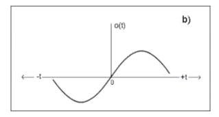
Odd signals are those signals which are asymmetrical in nature and are not identical at the origin. Mathematically, an odd signal must satisfy the following condition
