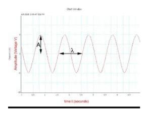
Deterministic signals are those signals which can be completely specific in time. This pattern of this type of signals is regular and can be characterized mathematically. In this ,the nature and amplitude of such a signal can be predicted.
