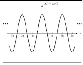
A signal x(t) is a continuous -time signal if t is a continuous variable. This means that signal is defined continuously in time domain.
