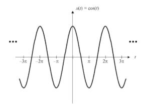
Even signals are those signals which exhibits symmetry in time domain and are identical are about the nature. Mathematically, an even signals must satisfy the following condition x(t)=x(-t)
