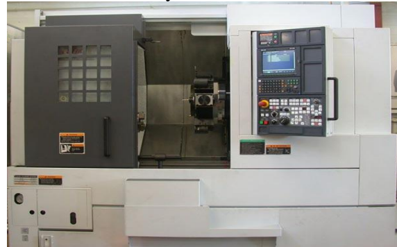
Fig: 4-axis CNC MORI SEIKI turning machine
