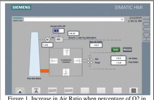
Figure 1. Increase in Air Ratio when percentage of O2 in stack is less than the set point
