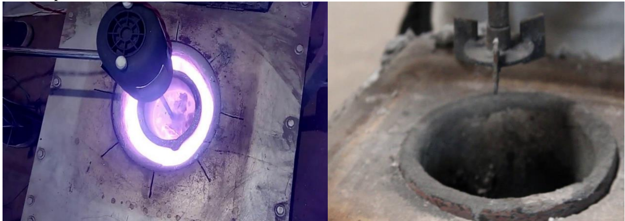
Fig – stir casting process
