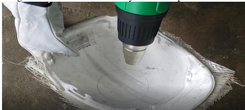
Fig Heat application with the help of hot air blower for removing dummy
