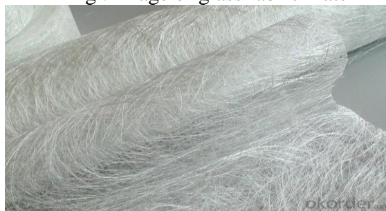
Fig: Image of Random oriented glass fiber
