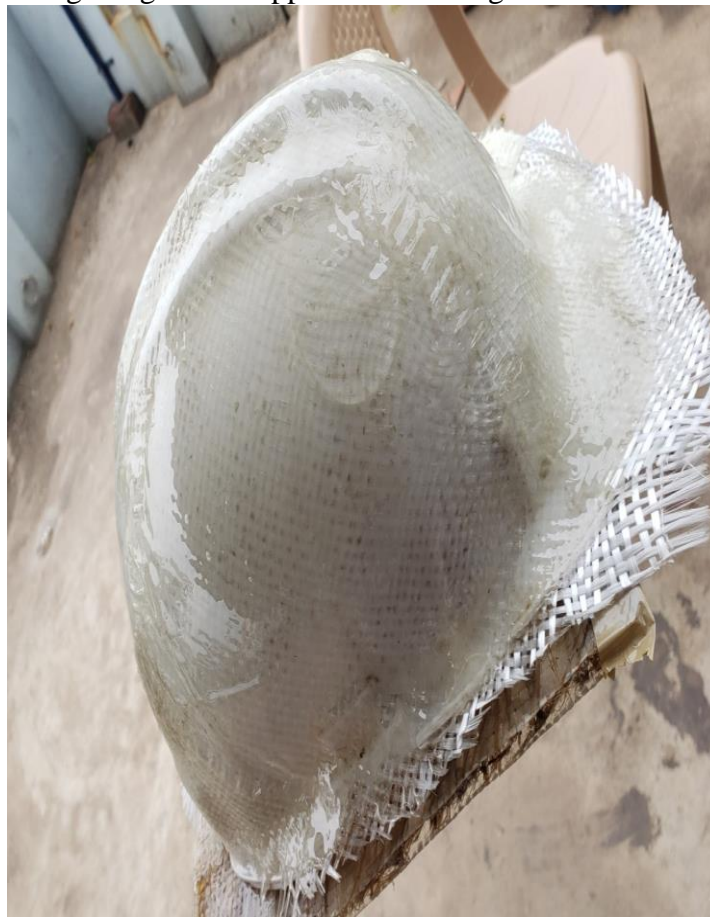
Fig Images after application of resign on fiber
