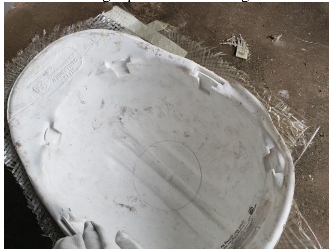
Fig: PVC helmet used as dummy inside the specimen
