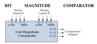
Some commercially available digital comparators such as the TTL 74LS85 or CMOS 4063 4-bit magnitude comparator have additional input terminals that allow more individual comparators to be "cascaded" together to compare words larger than 4-bits with magnitude comparators of "n"-bits being produced. These cascading inputs are connected directly to the corresponding outputs of the previous comparator as shown to compare 8, 16 or even 32-bit words
