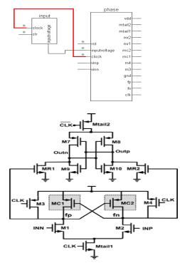
**Design of Dynamic Clocked Comparator** Comparator is the basic building block for the ADC applications. This application module developed consists of a single-tail this comes under the clocked regenerative comparator that can make fast decisions with the positive feedback. The main parameters considered here are the clock inputs and with this the double tail comparator is developed.
