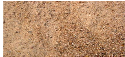
Figure 3.3 River sand used in concrete mixes
