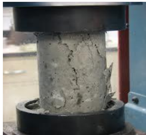
Cylinder under loading in UTM Cylinder after crushing
