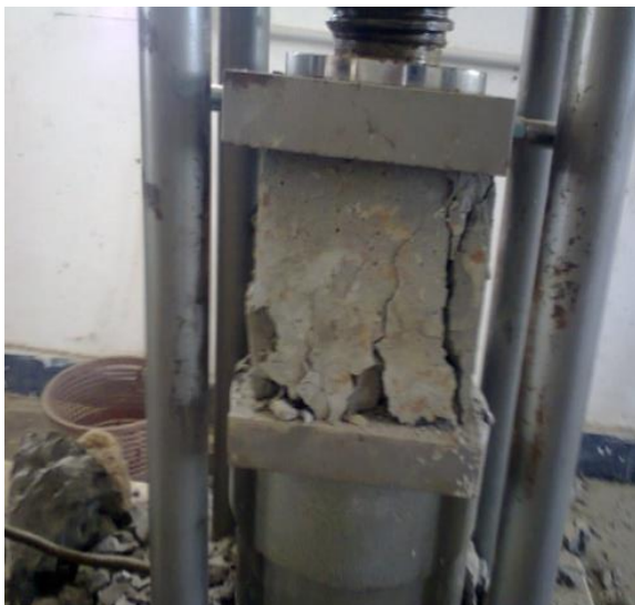
Fig:-4.10.1 Compressive strength of cube before testing and after testing
