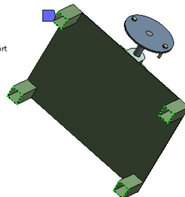
Figure.4 Boundary Condition of NVH Test Rig
