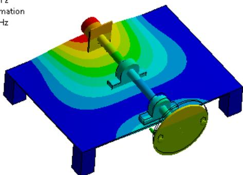
Figure.6 Total deformation of NVH Test Rig mode 2
