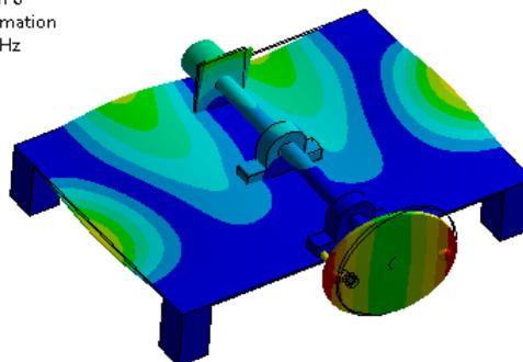
Figure.10 Total deformation of NVH Test Rig mode 6
