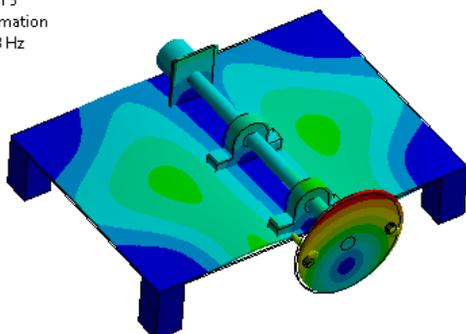
Figure.7 Total deformation of NVH Test Rig mode 3
