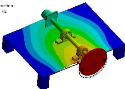
Figure.5 Total deformation of NVH Test Rig mode 1
