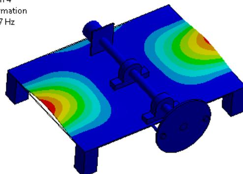
Figure.8 Total deformation of NVH Test Rig mode 4
