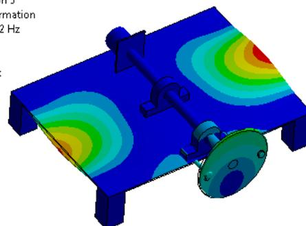
Figure.9 Total deformation of NVH Test Rig mode 5
