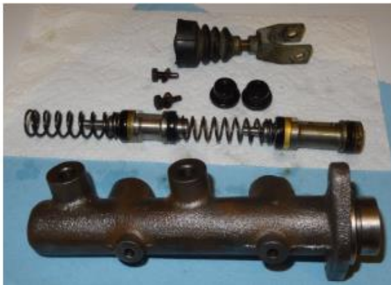
Fig: 1.5 Shows the twin pistons in master cylinder
