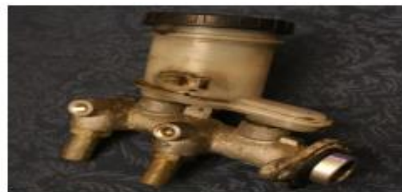
Fig: 1.1 shows the master cylinder model
