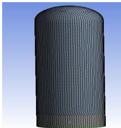
Meshing of composite radome
