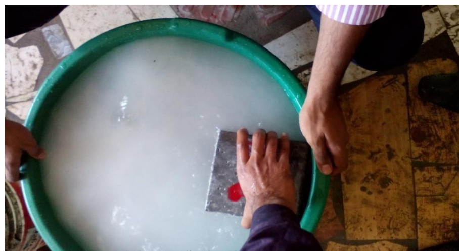
FIGURE 5.6: ALKALINE ATTACK TEST OF CONCRETE CUBES TABLE: 5.6% LOSS OF WEIGHT REDUCTION OF CUBES AFTER 28DAYS
