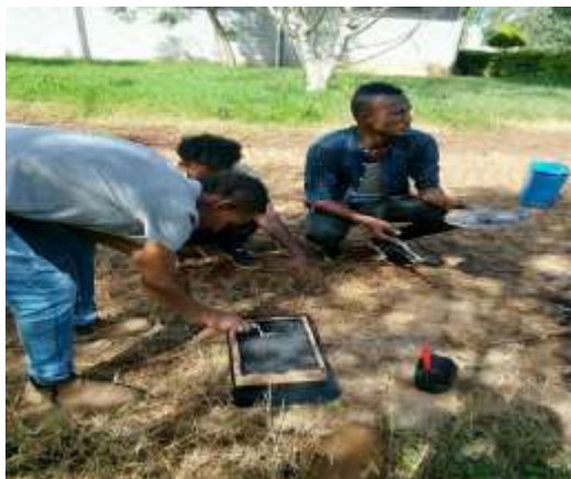
Figure 4 Casting into the Mold
