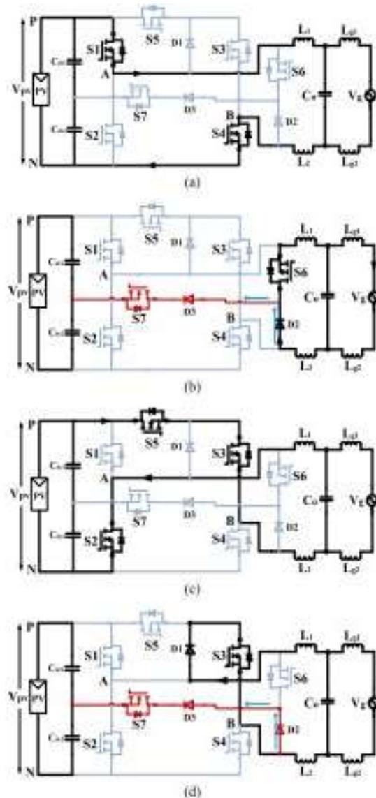
operation period. Therefore, the proposed topology could be implemented utilizing MOSFET switches. However, the body diode will be activated if a phase shift is occurred in the inverter output voltage and current. Accordingly, the dependability of the system will be reduced because of the MOSFET antiparallel diode low reverse-recovery issues.
