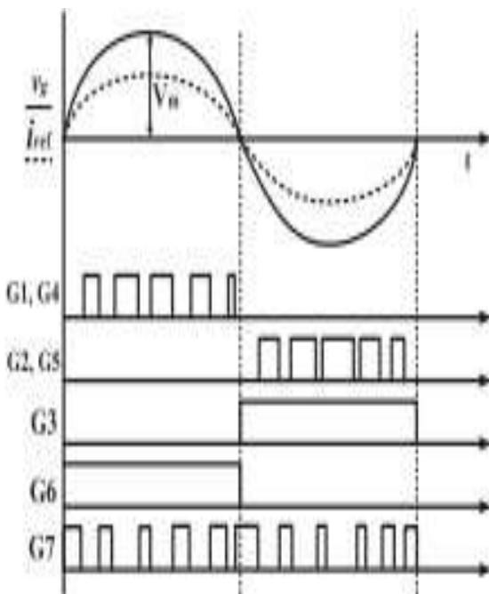
Fig 2.1: Gate drive signals of the proposed topology for the circuit structure A.
