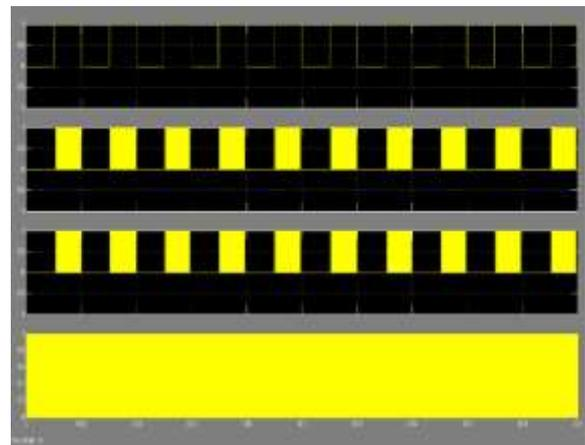
Fig 3.1.b Gate pulses for switching S<sub>1</sub>, S<sub>4</sub>, S<sub>6</sub> and S<sub>7</sub> switches.
