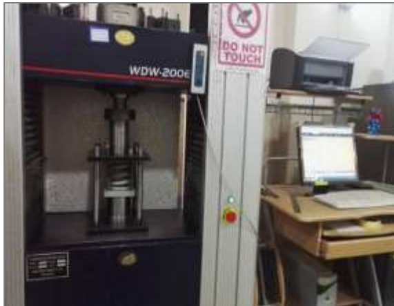
Figure 5: RPSMF die mounted to computerized testing machine.
