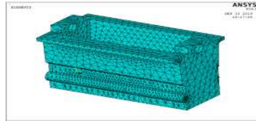
Fig.13 shows the meshed model of Engine block
