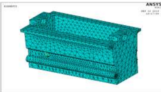
Applied fixed condition at bottom of engine block
