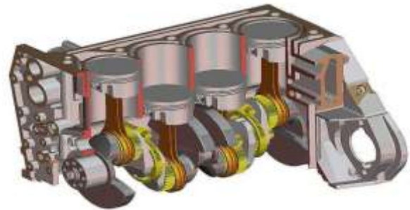
Fig.2 shows Monobloc cylinder block and crankcase
