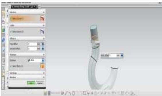
Fig.5.5 Sweep along 2D sketch of modified crane hook
