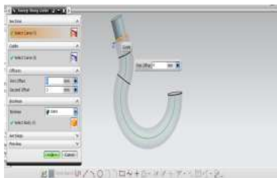
Fig.3.5 Sweep along 2D sketch of crane hook
