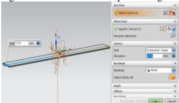
Fig: shows the 3D extrusion of the spoiler wing
