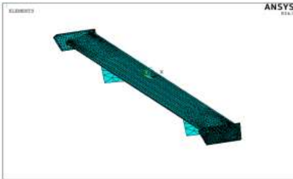
Fig. Created mesh on spoiler
