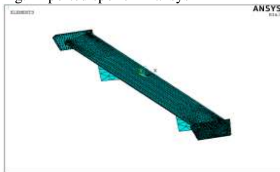
Fig. Created mesh on spoiler
