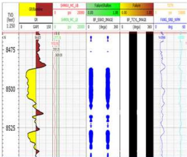
**Figure 1: A cut section of the TVD, lithology, maximum and minimum horizontal stress, failure image and friction angle logs.**
