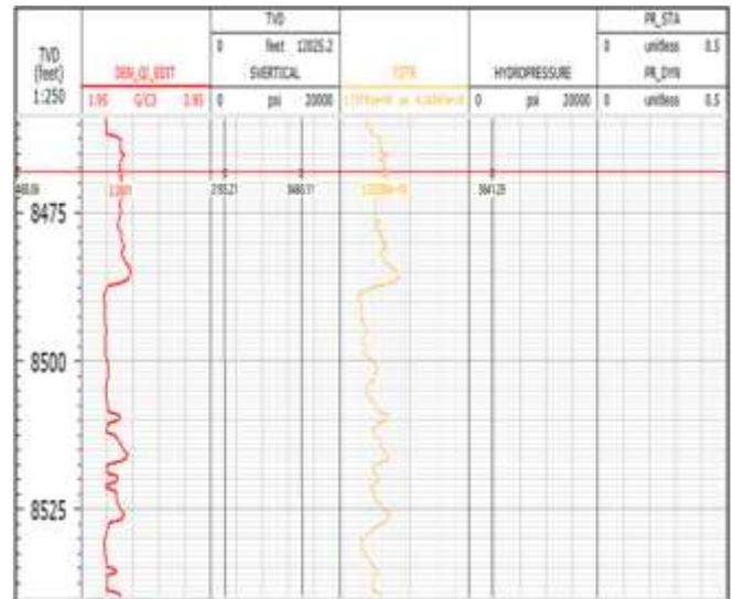
**Figure 2: A cut section of the TVD, density, vertical stress, tensile stress, hydrostatic pressure, static and dynamic Poisson ratio logs.**
