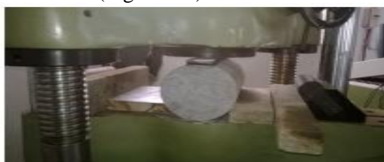
FIGURE 4.2 SPLIT TENSILE TEST
