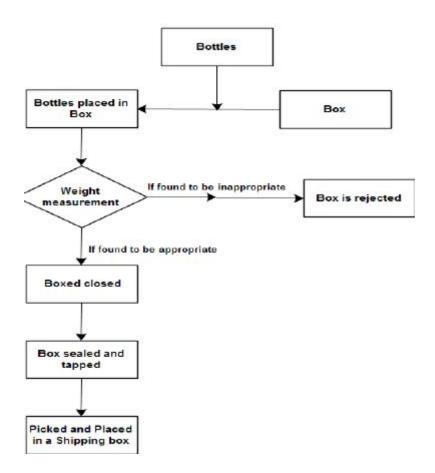
The above diagram show the flow of steps that we follow in the procedure first the bottles will be placed in a box then it will goes to the weight measurement if found to be inappropriate the box will be rejected or if the box weight found appropriate the box will be closed then the box will be sealed and tapped then picked and placed in a shipping box then it will go to the storage.
