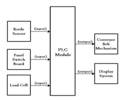
The above Block diagram shows that Bottle sensor panel switch board and Load cells are internally connected the outputs are conveyor belt Mechanism and Display system shows how does the controllers are actually connected. Generally the sensors that we will use are inductive sensors and switches that we will use are limit switches and mostly pushbuttons.
