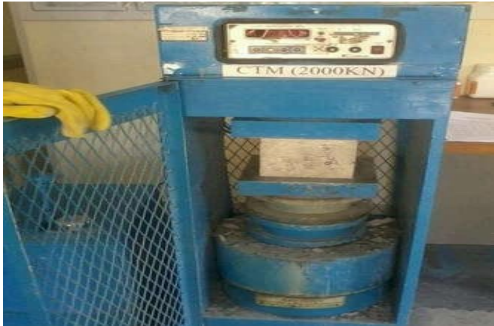
Fig. 1 Compression strength test set up
