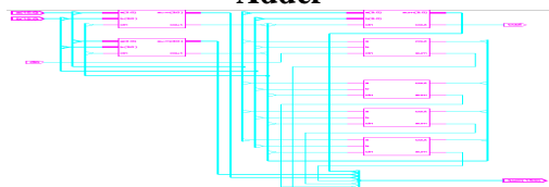
Figure 7.3.7 : Internal block of Carry-Select Adder
