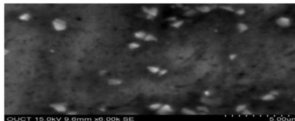
Fig: SEM Image OF AA7050 with 5% Wt. of Silicon carbide
