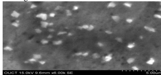
Fig: SEM Image of AA7050 with 15% Wt. of Silicon carbide
