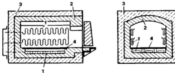
Fig: Indirect Resistance Heat Chamber Furnace
