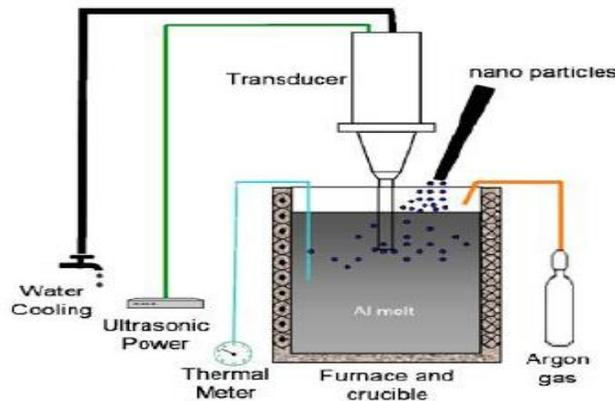
Fig: Schematic diagram of Experimental setup
