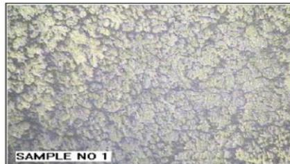
Fig: Microstructure of Raw AA7050
