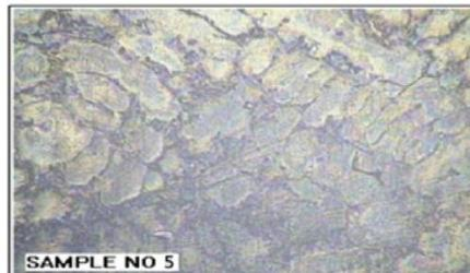
Fig: Microstructure of AA7050 with 20% Wt of Silicon carbide
