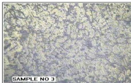
Fig: Microstructure of AA7050 with 10% Wt of Silicon carbide
