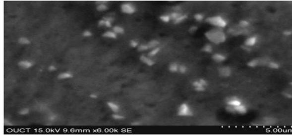
Fig: SEM Image of AA7050 with 10% Wt. of Silicon carbide
