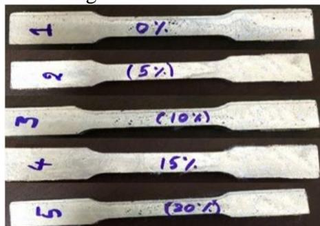
Fig: Al Cast Alloy According To ASTM E8 Standards
