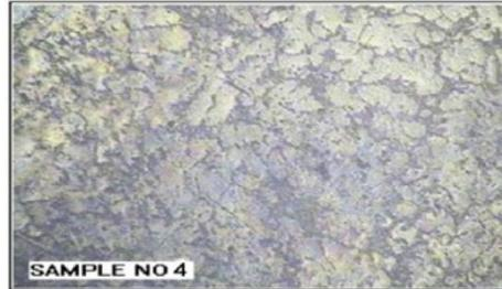
Fig: Microstructure of AA7050 with 15% Wt. of Silicon carbide
