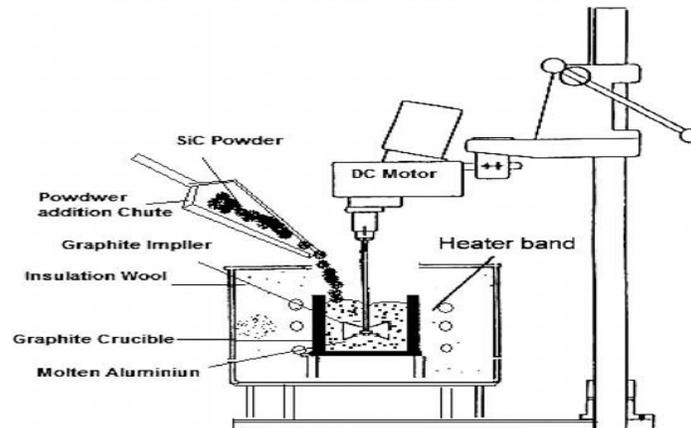
Fig: Layout of the stir casting apparatus
