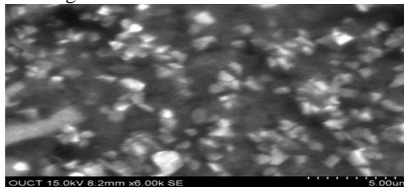
Fig: SEM Image of AA7050 with 20% Wt. of Silicon carbide
