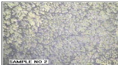
Fig: Microstructure of AA7050 with 5% Wt of Silicon carbide
