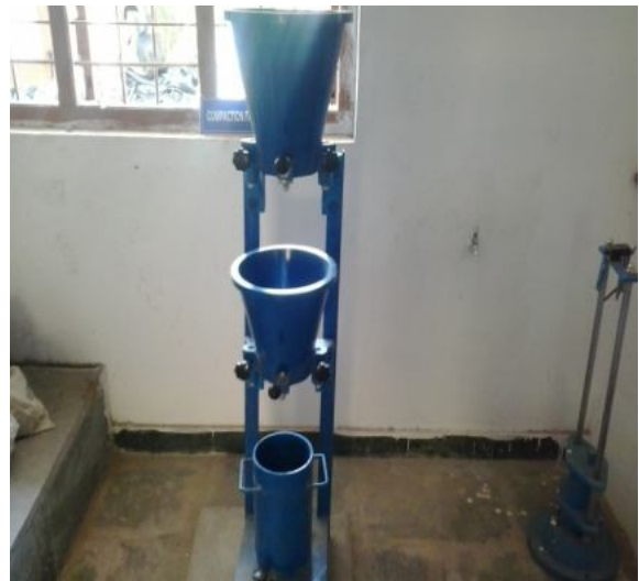
Fig 4.9.1 compaction factor apparatus
