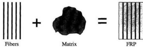
Fig. 3.1 Formation of Fiber Reinforced Polymer Composite
