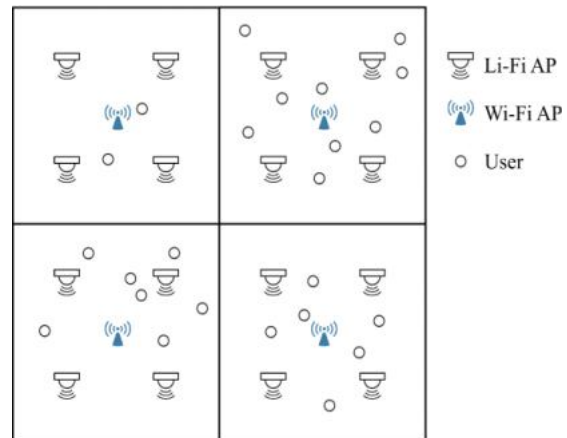
Fig. 1 Schematic diagram of an indoor hybrid Li-Fi and Wi-Fi network.
