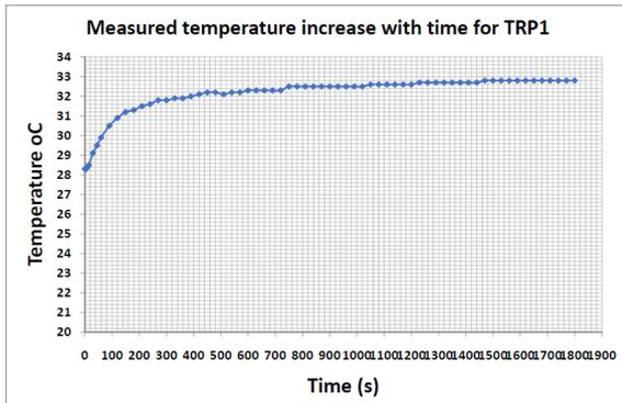
Figure 3 : Graph of Temperature oC versus Time (s) for TRP1. Calculated Thermal Resistivity value of 0.295466206 °Cm/W.
