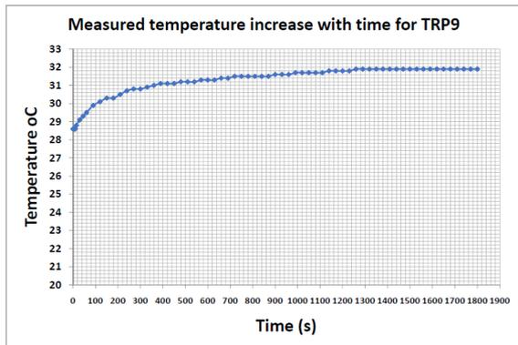
Figure 11: Graph of Temperature oC versus Time (s) for TRP9. Calculated Thermal Resistivity value of 0.309289523 °Cm/W.
