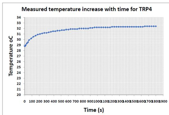
Figure 6: Graph of Temperature oC versus Time (s) for TRP4. Calculated Thermal Resistivity value of 0.298742062 °Cm/W.
