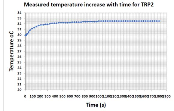
Figure 4 : Graph of Temperature oC versus Time (s) for TRP2. Calculated Thermal Resistivity value of 0.151973588 °Cm/W.
