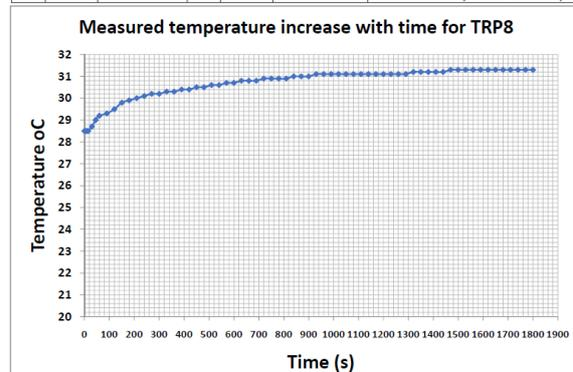
Figure 10: Graph of Temperature oC versus Time (s) for TRP8. Calculated Thermal Resistivity value of 0.229950673 °Cm/W.
