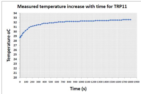
Figure 13: Graph of Temperature oC versus Time (s) for TRP11. Calculated Thermal Resistivity value of 0.233716731 °Cm/W
