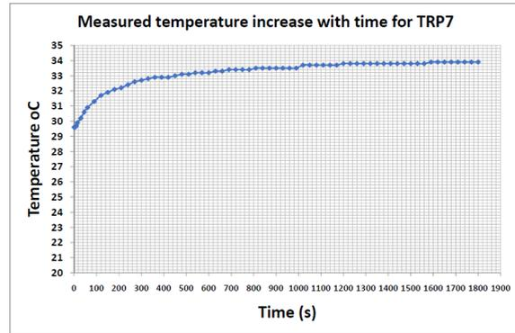
Figure 9: Graph of Temperature oC versus Time (s) for TRP7. Calculated Thermal Resistivity value of 0.306219671 °Cm/W.
