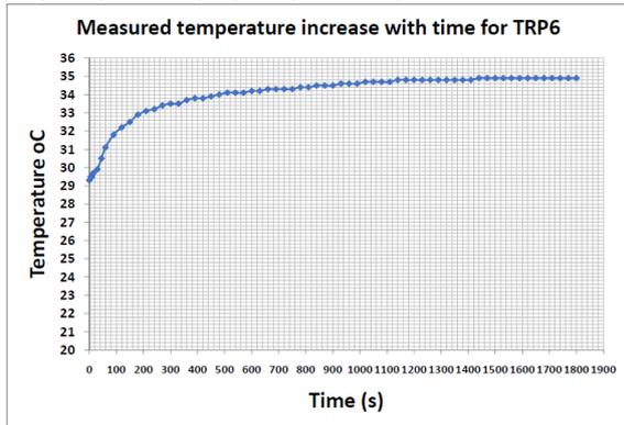
Figure 8: Graph of Temperature oC versus Time (s) for TRP6. Calculated Thermal Resistivity value of 0.455356332 °Cm/W.
