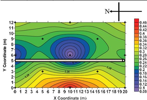
Figure 16: Thermal resistivity distribution model within a grid, with a hypothetical pipeline placed across.
