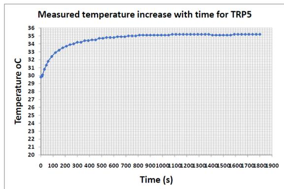
Figure 7: Graph of Temperature oC versus Time (s) for TRP5. Calculated Thermal Resistivity value of 0.075798824 °Cm/W.
