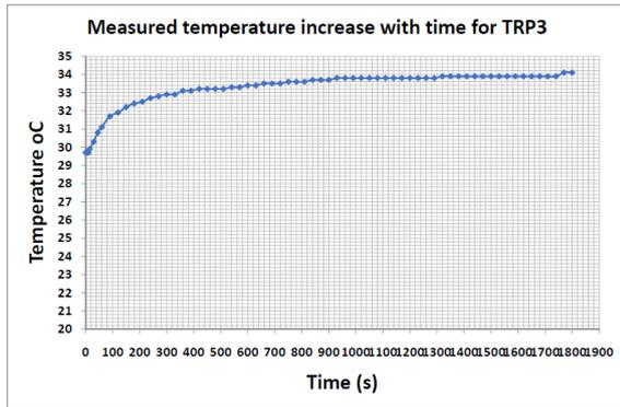
Figure 5: Graph of Temperature oC versus Time (s) for TRP3. Calculated Thermal Resistivity value of 0.30021551 °Cm/W.
