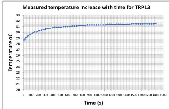
Figure 15: Graph of Temperature oC versus Time (s) for TRP13. Calculated Thermal Resistivity value of 0.23138831 °Cm/W
