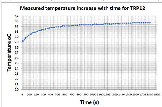
Figure 14: Graph of Temperature oC versus Time (s) for TRP12. Calculated Thermal Resistivity value of 0.312798611 °Cm/W.
