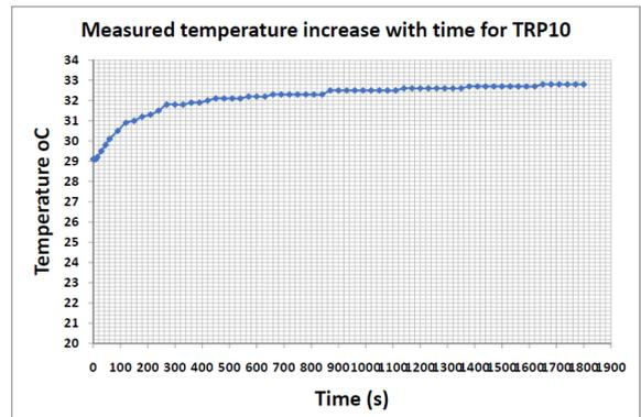
Figure 12: Graph of Temperature oC versus Time (s) for TRP10. Calculated Thermal Resistivity value of 0.313586516 °Cm/W.
